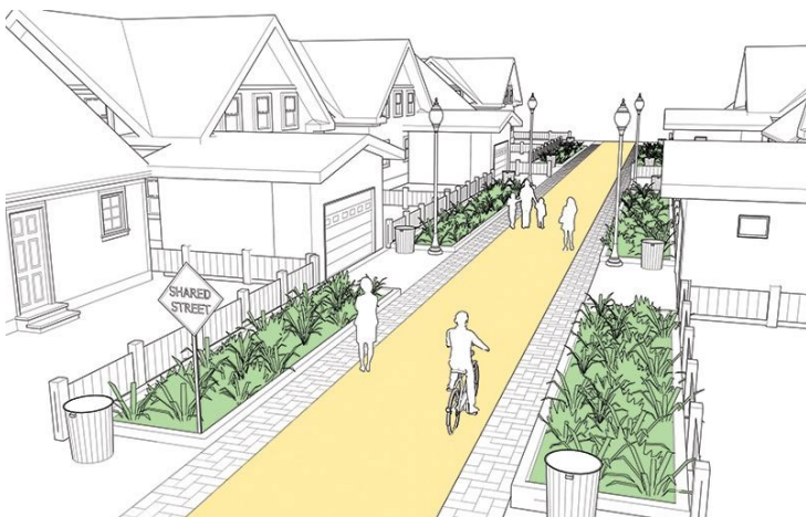
Figure 5-1. Example of a green alley. Retrofitted alleyways provide an opportunity to revive a residential area and integrate it more meaningfully as a community-building asset. Important features include low impact pavement, human-scale lighting, rain gardens on the periphery and shared street design to accommodate residential vehicles, pedestrians, and cyclists as well as service and utility vehicles [6].
