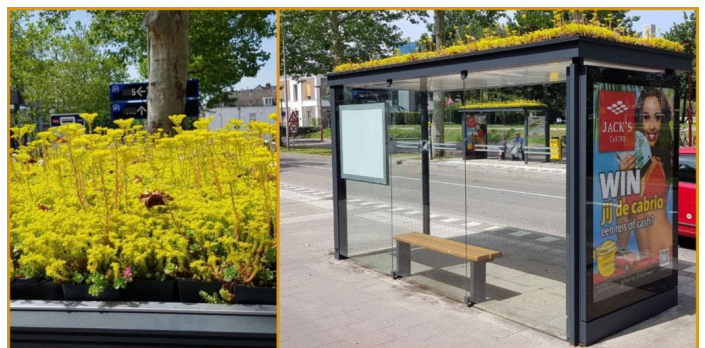
Figure 5-9. Green bus shelters. The Dutch City of Utrecht deployed bee sanctuaries on 315 bus stops to help encourage pollination, help regulate temperatures, reduce PM2.5 content in the air near the bus stops, and capture fine dust and store rainwater at their bus shelter locations. The City of Utrecht selected a low maintenance family of grass and wildflowers called sedum plants, which required very little water [37].
