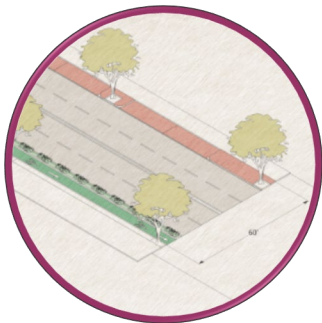
Figure 4-10. Primary Corridor design typologies are an appropriate choice to retrofit minor arterials and collector streets. Green protected bike lanes and soil cells to support urban tree growth can help transform these into multimodal connectors.
