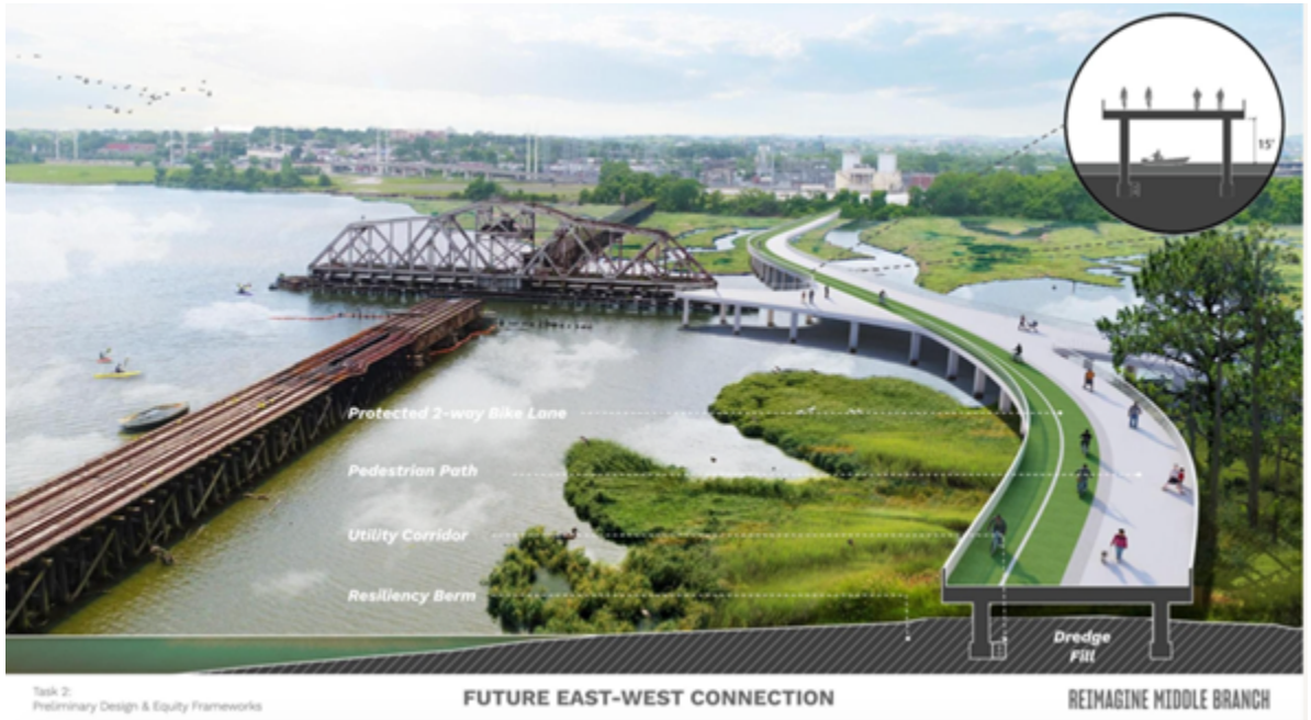
The Plan envisions a new east-west bridge connecting Westport and Mount Winans to Port Covington and the South Baltimore peninsula. The design includes bike and pedestrian lanes, and integrates wetlands and resiliency berms to protect nearby neighborhoods from flooding, while continuing to enable boats to access Ridgely’s Cove. Credit: James Corner Field Operations.
